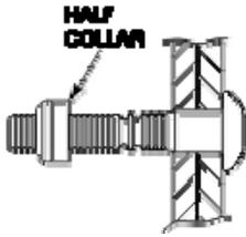
**Half Collar:** A reduced height lock bolt collar used to minimize collar protrusion. Note: will reduce tensile performance. Compare to full collar.
